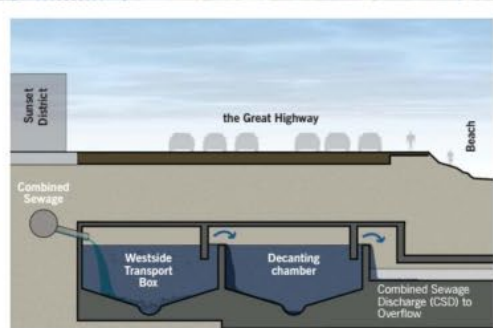
Figure III-6: Westside Transport Box Sectional Diagram (at overflow decanting station)
